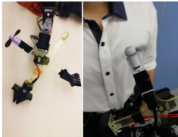
Figure 57 integrating multiple types of sub-end effectors can contribute to increasing the robot's uses
