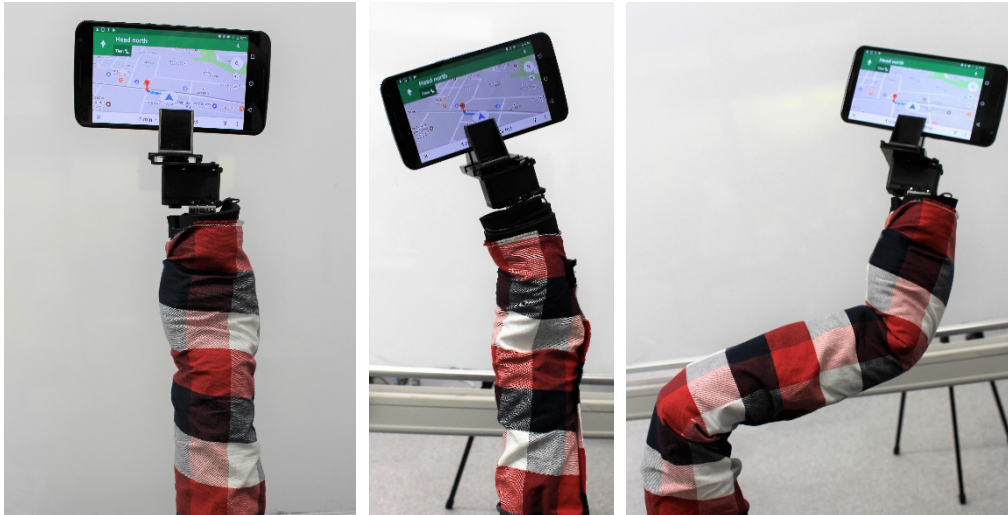
Figure 54 A navigation application is developed, which demonstrates how a serpentine-shaped wearable appendage can be used to amplify the interaction capabilities of a smartphone. In the pictures, the robot automatically leans in various directions to indicate where the user should be heading based on navigation information.
