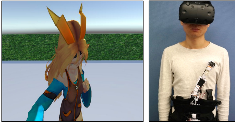
Figure 22 the idea of HapticSerpent is to investigate novel haptic feedback in VR. For example, within a VR experience, if the user is punched by the VR character (Left) the robot can simultaneously deliver feedback with matching physical properties (Right), such as strength, speed, angle of contact or location.
