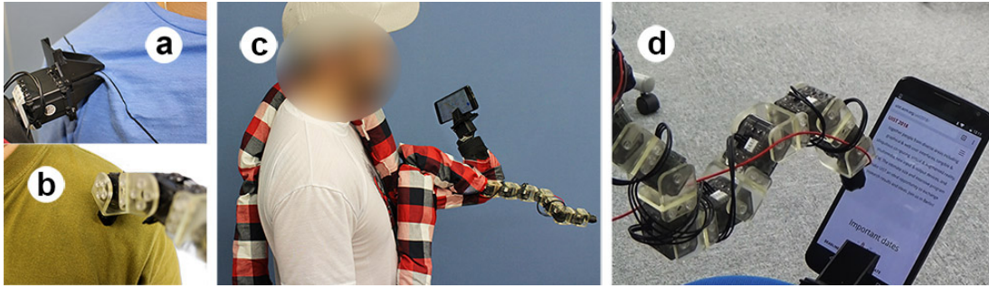
Figure 16 a,b) Orochi can deliver a haptic feedback in different locations and c,d) augment interactions with digital devices, such as a smartphone, in different ways.
