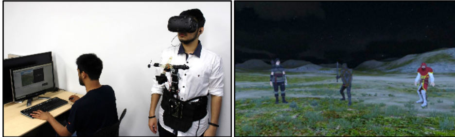
Figure 44 1) User study conditions and hardware. We utilized HTC Vive to deliver our VR experience. Two PCs were used, one for running Unity3D/VR experience, and the other to control the robot. 2) The VR environment involves several experiences with changing weather, ambient effects and day/night cycles.
