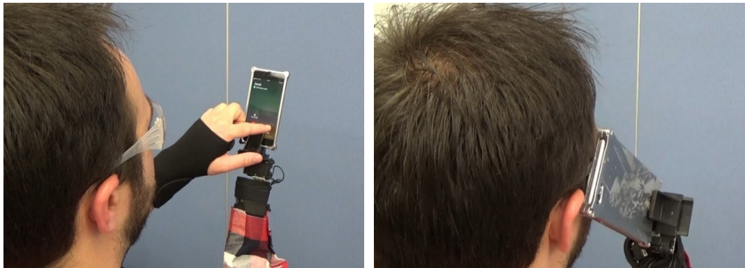
Figure 53 (left) when the user selects to answer the phone call, (right) the robot automatically brings the phone to his head to talk. In this scenario, Orochi augments the smartphone with actuation capabilities, which can be used to develop enhance trivial smartphone applications.
