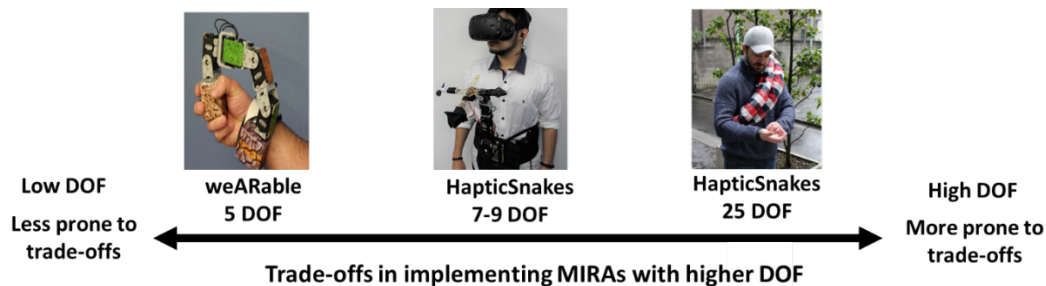
Figure 61 trade-offs with relation of DOFs. Based on our the case studies that were implemented using servomotors, the higher DOFs, the more prone a wearable to various trade-offs.
