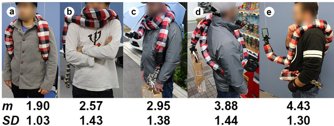
Figure 19 Orochi’s noticeability ratings in each context, The low ratings in (a,b) show that Orochi is mostly unnoticeable when retracted, and more noticeable when used (c,d,e).
