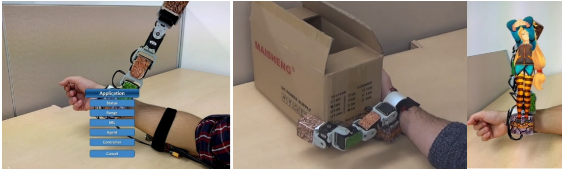
Figure 51 (Left) the AR menu allows the user to control intrinsic attributes and access/exit various modes of operation and experiences. (Middle) Users can select various poses and actions from the AR menu to support different physical manipulation needs. (Right) The companion character can provide auditory, shape-shifting and haptic interaction experiences.
