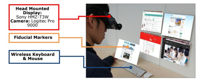
Figure 5: A participant using our prototype with fiducial markers on the wall and in the user's hands.
