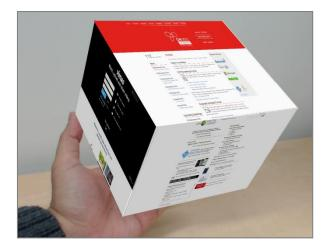
**Figure 9**: A physical cube-shaped object that is textured with web pages in each side (with AR). Users can physically rotate or manipulate the cube to view different webpages in every side.
