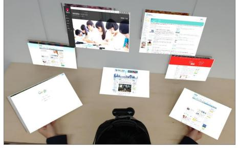
**Figure 6:** A user physically manipulating position, orientation and proximity attributes of fiducial markers with his hands. The fiducal markers' attribute-changes are simultaneously applied to web pages in AR.
