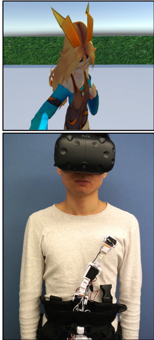
Figure 1: (Upper) A user is being punched in the chest in VR. (Lower) A haptic force with similar magnitude and location is applied to his chest through the HapticSerpent arm.
