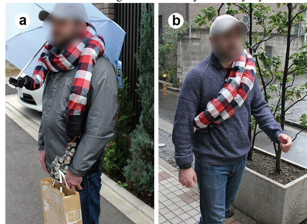
Figure 1 Orochi is a multipurpose SRL that a) can be worn and used across daily contexts and b) is unobtrusive in public.
