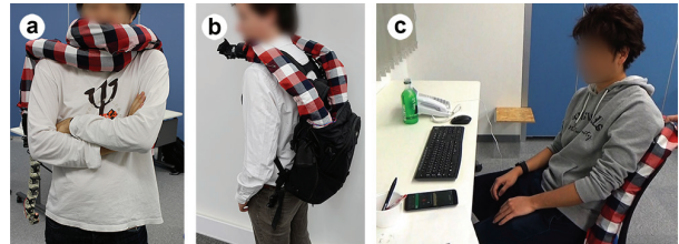
Figure 8 a) One participant preferred wearing Orochi as a scarf that automatically covers his face when it is cold. b) One participant placed it in a backpack, and another c) around his seat, doubling as back support and to retrieve objects.
