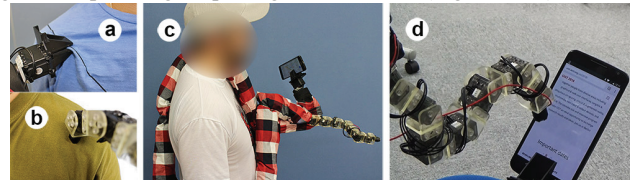
Figure 7 a,b) Orochi can deliver a haptic feedback in different locations and c,d) augment interactions with digital devices, such as a smartphone, in different ways.
